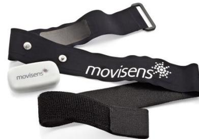
Figure 4: Activity + ECG-Sensor (EcgMove 3 with chest belt)
